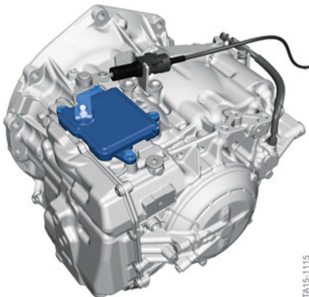
F48 EGS, 8-speed automatic transmission
